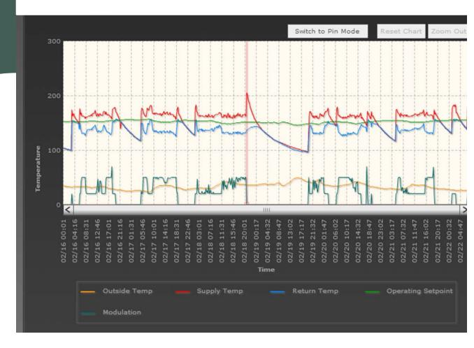
Night setback has huge value benefits to energy reduction and boiler operation. Think about it, what happens at night? Temperature outside drops, water temperature therefore rises and the BMS has the room stats in a setback mode ultimately at the near closed position. Why heat water up when the building is unoccupied. Let the water temperature cool the space.
